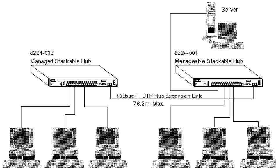
Figure 26. Interconnecting 8224 Hubs via the Hub Expansion Ports
