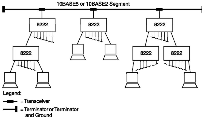
Figure 19. 8222 Hubs in a Network with Coaxial Segments
