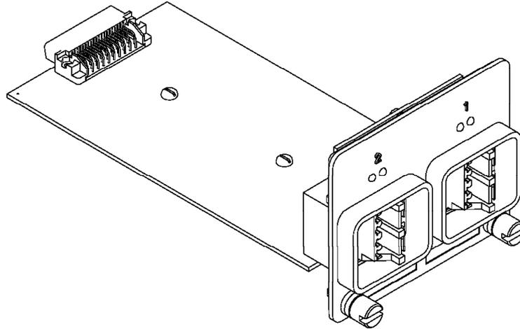
Figure 48. ICS Lobe Insertion Unit (LIU) Module
