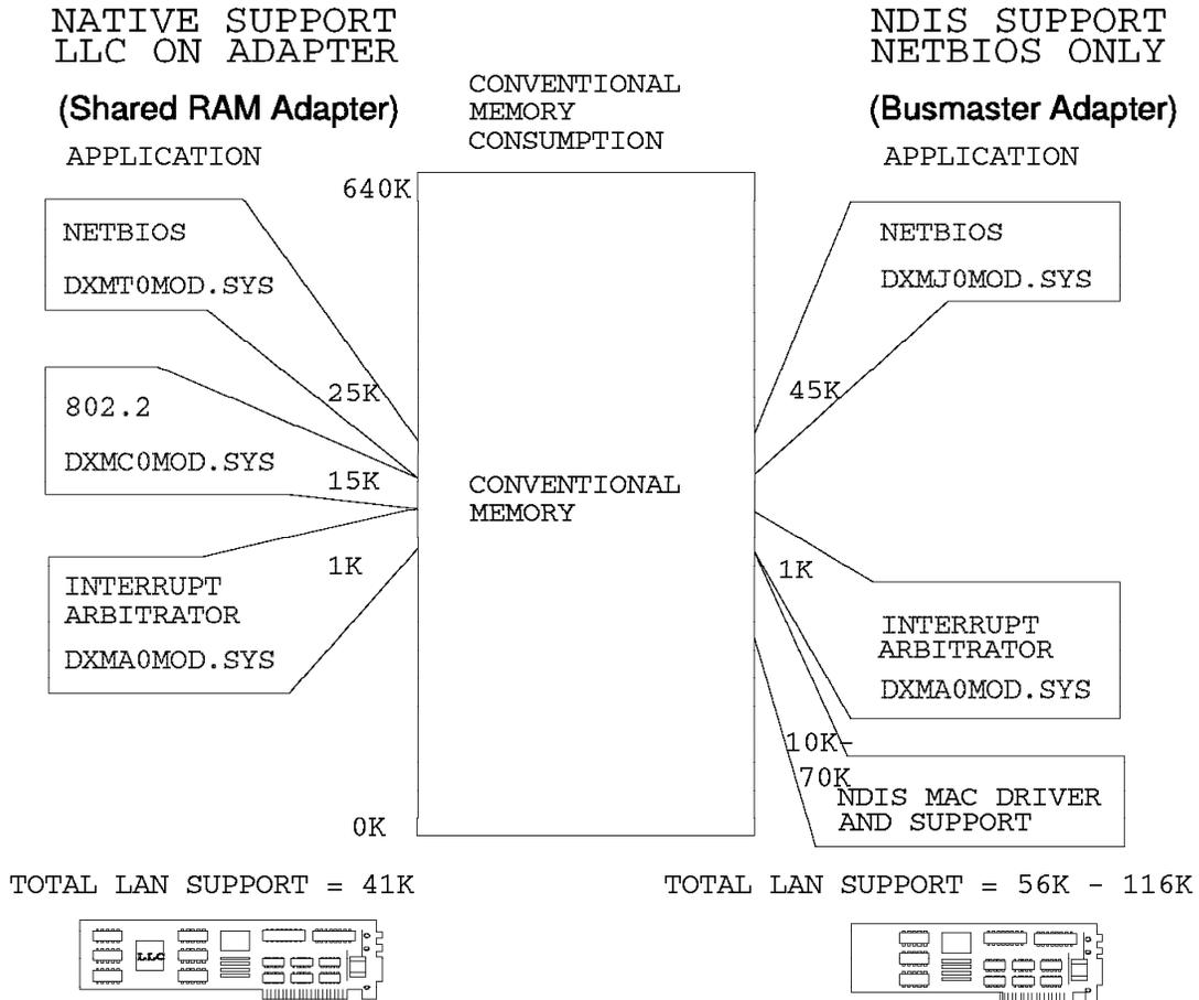
Figure 12. LSP DOS Memory Consumption with J0 Module
