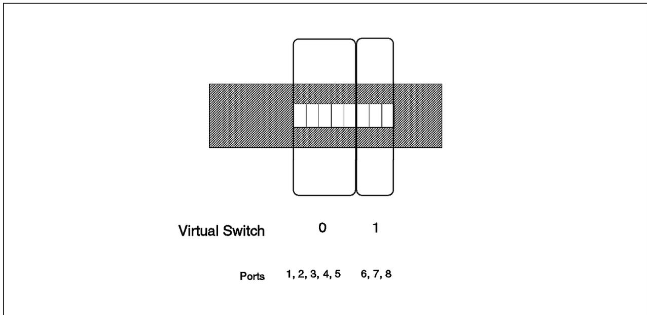
Figure 103. Switch Divided in Two Using TokenPipe
