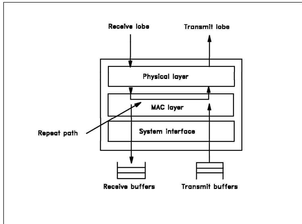
Figure 105. Normal Operation of a Token-Ring Adapter
