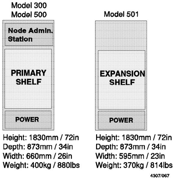
Figure 109. 2220 Nways Switch Rack Configuration
