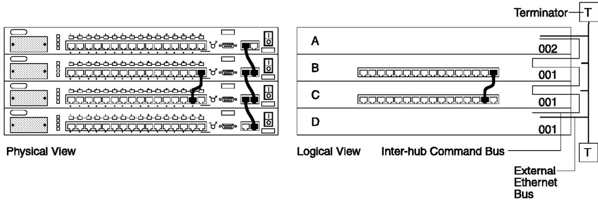
Figure 34. 8224 Hub C - Cascaded from Hub B
