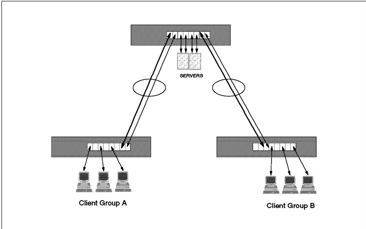
Figure 99. 8271 Connection Using EtherPipe
