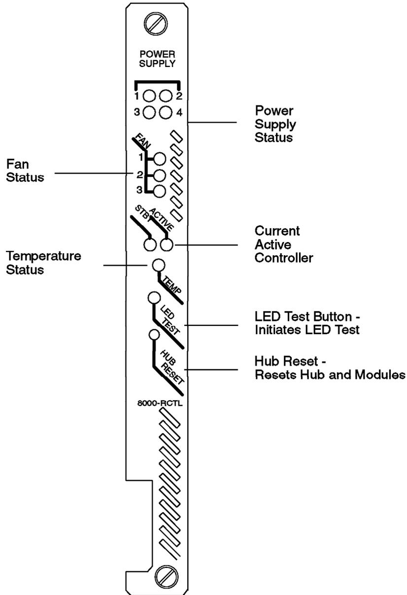
Figure 90. Front View of the Controller Module
