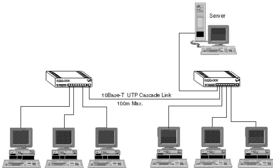
Figure 17. 8222 in a Typical IEEE 802.3 Network
