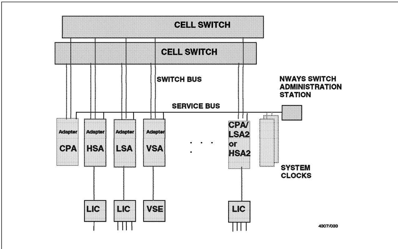
Figure 110. 2220 Nways Switch Hardware Components
