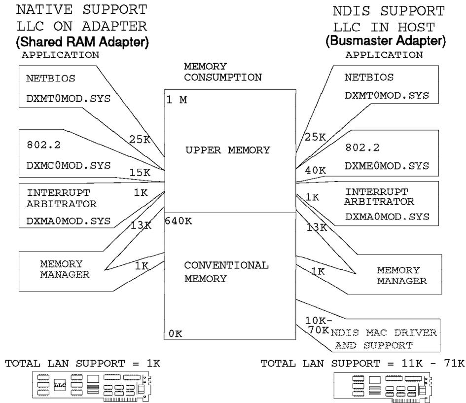
Figure 13. LSP DOS Memory Consumption Utilizing Upper Memory
