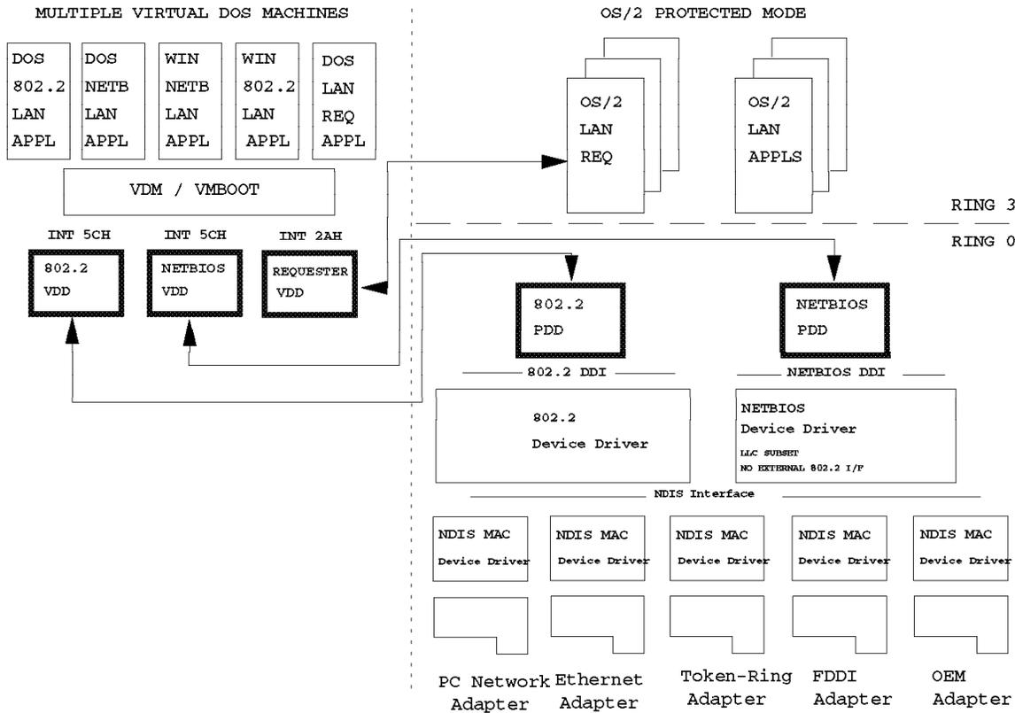
Figure 6. OS/2 NTS/2 Support for DOS LAN Applications
