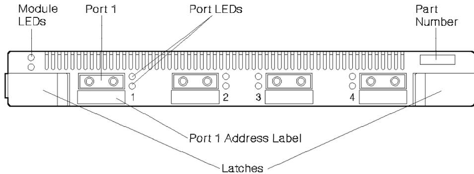
Figure 72. IBM 8240 Device Attachment Module for Optical Fiber
