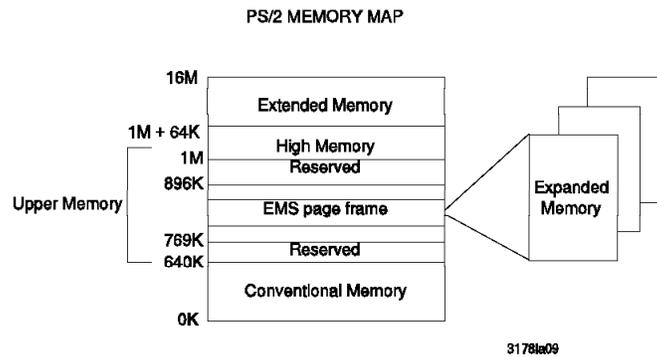
Figure 9. Memory MAP for DOS PS/2 Environments
