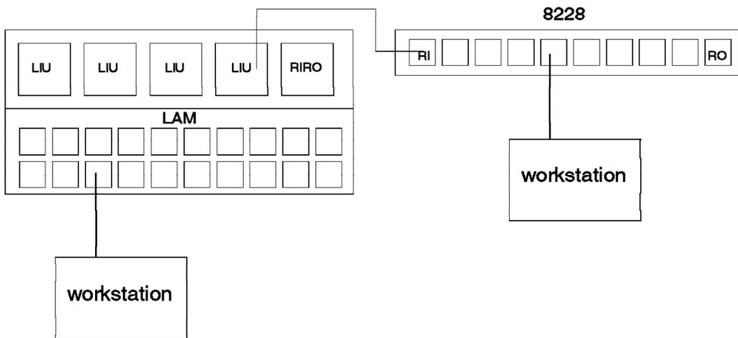
Figure 64. Fan-Out Using 8228s
