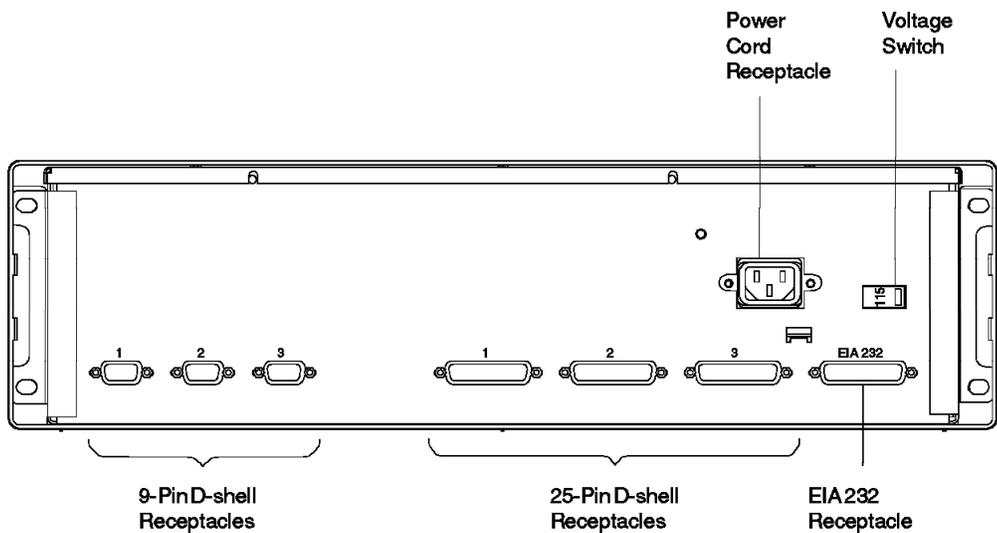
Figure 42. Rear View of an 8230-003/013
