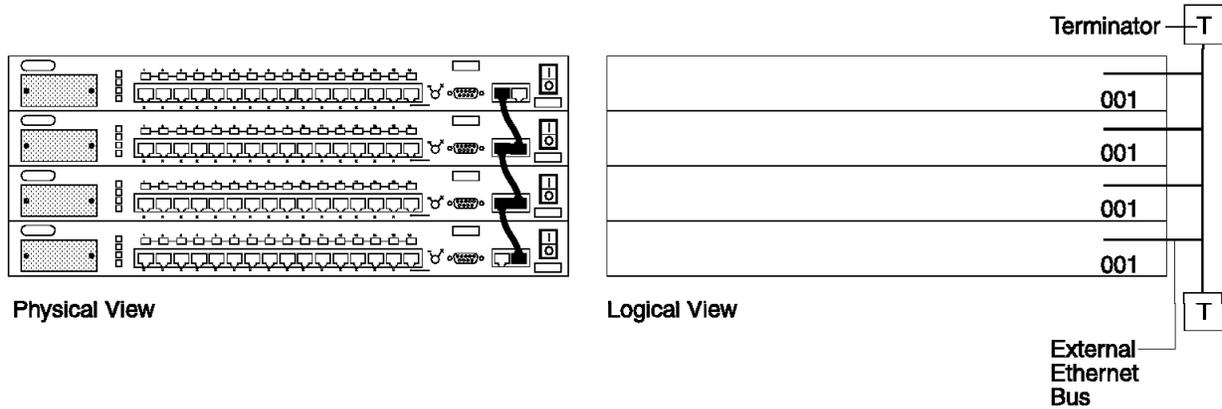
Figure 25. A Stack of Four 8224 Model 001s
