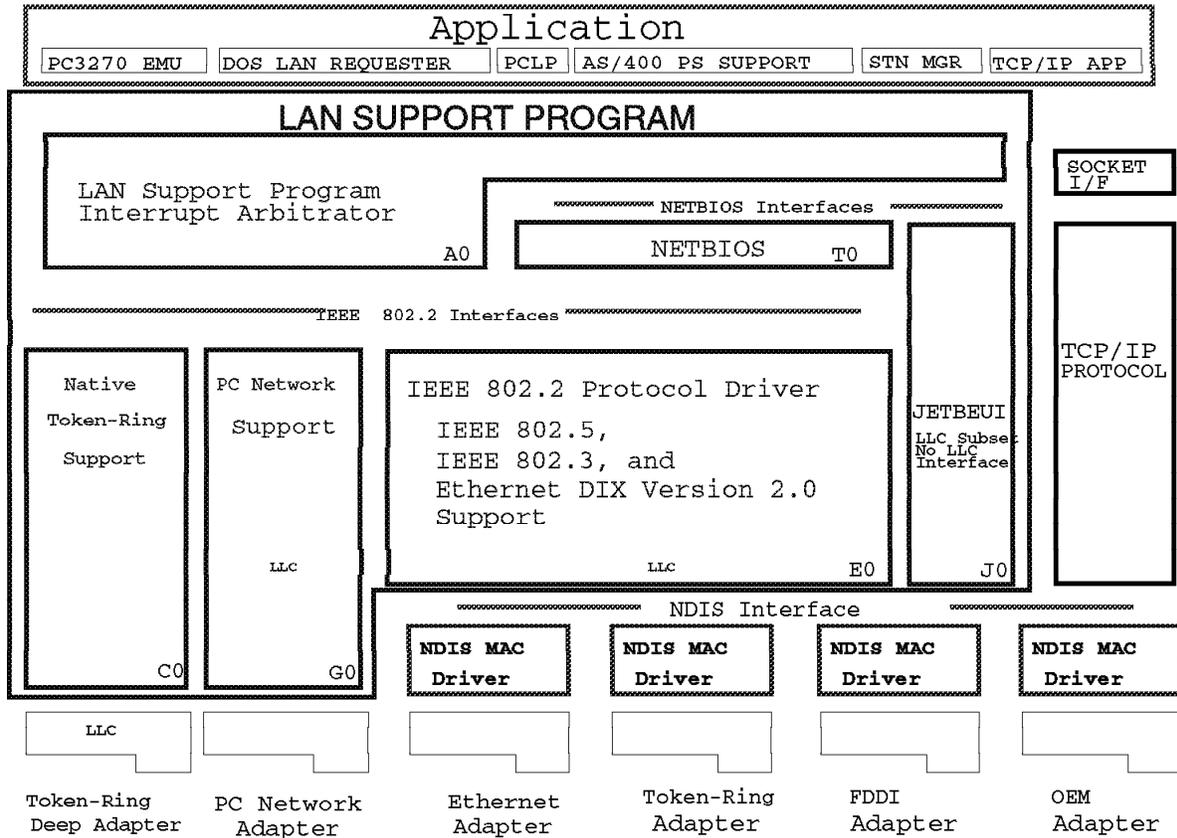
Figure 7. DOS Transport for IBM LAN Adapters
