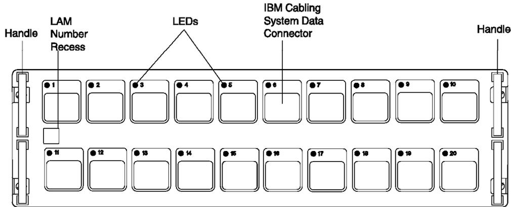
Figure 52. Front View, ICS Lobe Attachment Module (LAM)
