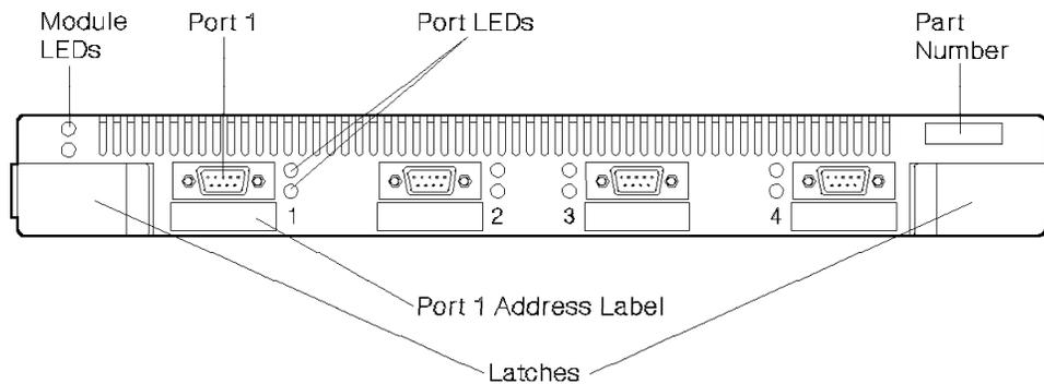
Figure 73. IBM 8240 Device Attachment Module for Copper
