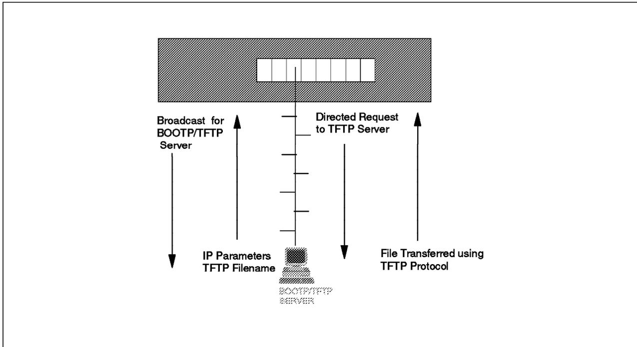
Figure 100. Communication between the BOOTP Server and the 8271
