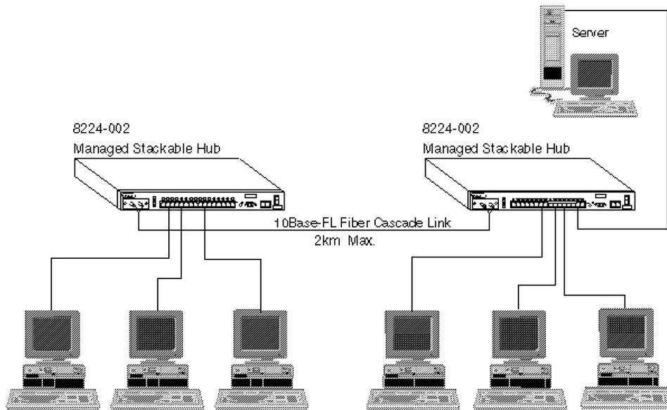
Figure 27. Cascading 8224 Hubs via Fiber Media Expansion Ports
