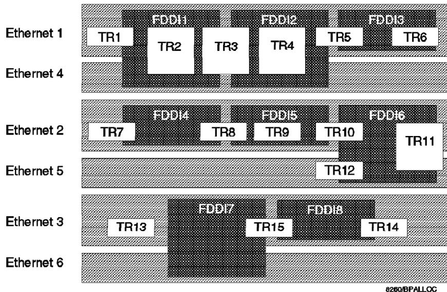
Figure 88. TriChannel Backplane Network Allocation
