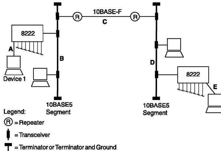
Figure 20. 8222 Hubs in a 10Base5 and Fiber Network
