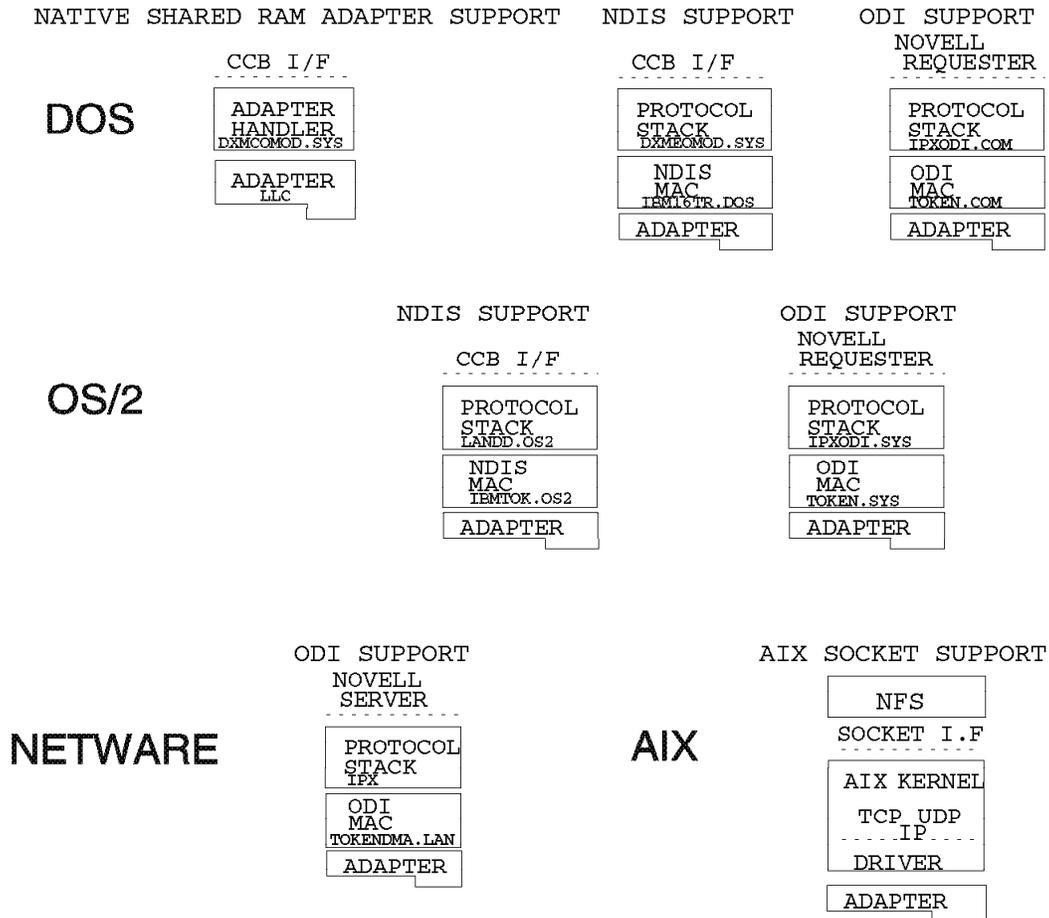
Figure 4. OS and Driver Environments with Module Name Examples
