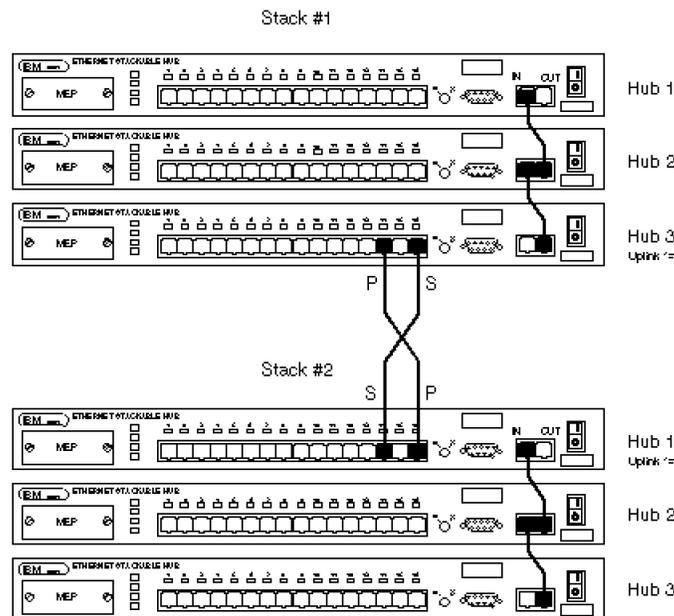
Figure 37. Two IBM 8224 Stacks - With Backup Ports Enabled - Cascading Application. This example shows multiple hub stacks connected via cascading over a backed-up 10Base-T link. The link between port 14 on hub 3 on stack 1 to port 16 on hub 1 of stack 2 is the primary (P) connection. The link between port 16 on hub 3 on stack 1 to port 14 on hub 1 of stack 2 is the secondary (S) or backup connection.
