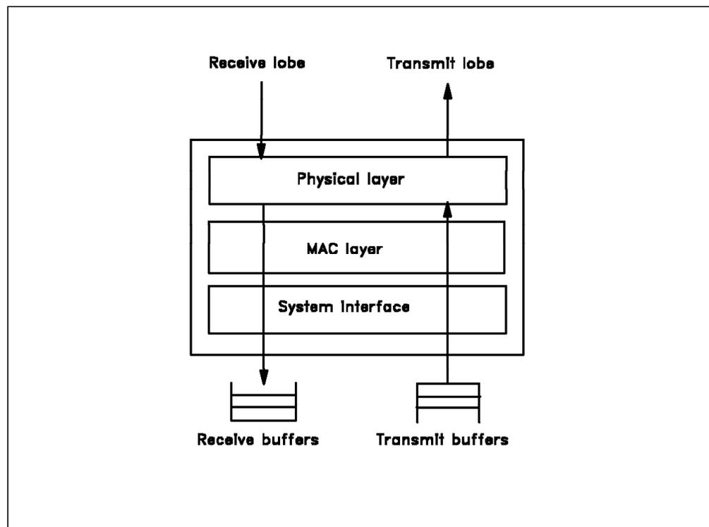
Figure 106. Full-Duplex Operation of a Token-Ring Adapter
